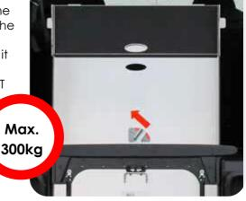
When the handle is pulled up, the ramp can be lowered. Mind that the ramp should rest on a flat surface. Otherwise it could bend when the wheelchair rides over it.
