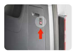
Pull the wheelchair out of the car (having the switch switched on) and detach the two belts on the front side of the wheelchair.
