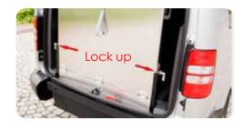
When having a foldable ramp, unlock the ramp with the two lockpins and be sure you fold the ramp carefully!
