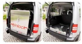
Push the handle down to fold the ramp.
