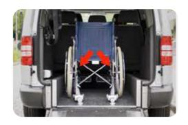
Disconnect the two retractors from the floor and place them in a safe place in the car.
