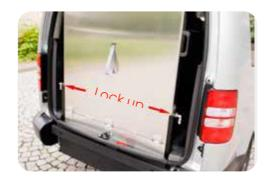
Close the tailgate. When closing it, the car automatically goes back to its original driving position. In cold situations (below 5°C) the gassprings tend to get harder, therefore close the tailgate gently in order not to bend the gassprings.
