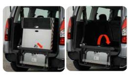
Close the tailgate. When closing it, the car automatically goes back to its original driving position. In cold situations (below 5°C) the gassprings tend to get harder, therefore close the tailgate gently in order not to bend the gassprings.
