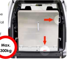
When the car is fully kneeled, the ramp can be lowered by pulling the handle to the top. Be aware that the ramp does not fall down when pulling the handle.
