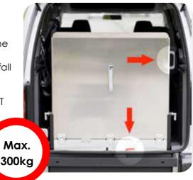
When the car is fully kneeled, the ramp can be lowered by pulling the handle to the top. Be aware that the ramp does not fall down when pulling the handle. Therefore, stop it with one hand.
