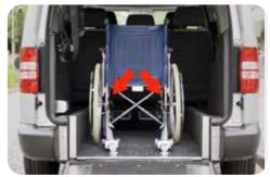
The belts have to be attached to the points which are marked at the rear of the wheelchair. If these points are not present, the belt has to be attached as high as possible, onto a vertical tube.
