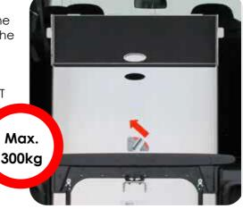
When the handle is pulled up, the ramp can be lowered. Mind that the ramp should rest on a flat surface. Otherwise it could bend when the wheelchair rides over it.
